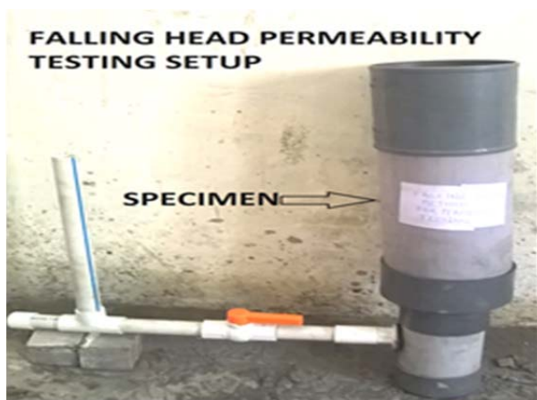
Fig. 1: Test setup of permeability test
